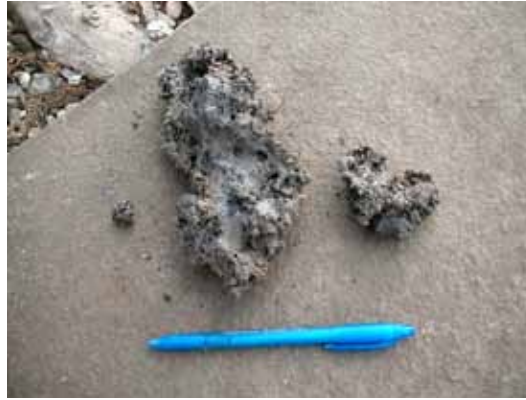
Typical ash “clinkers” formed during the combustion of 100% switchgrass pellets.
