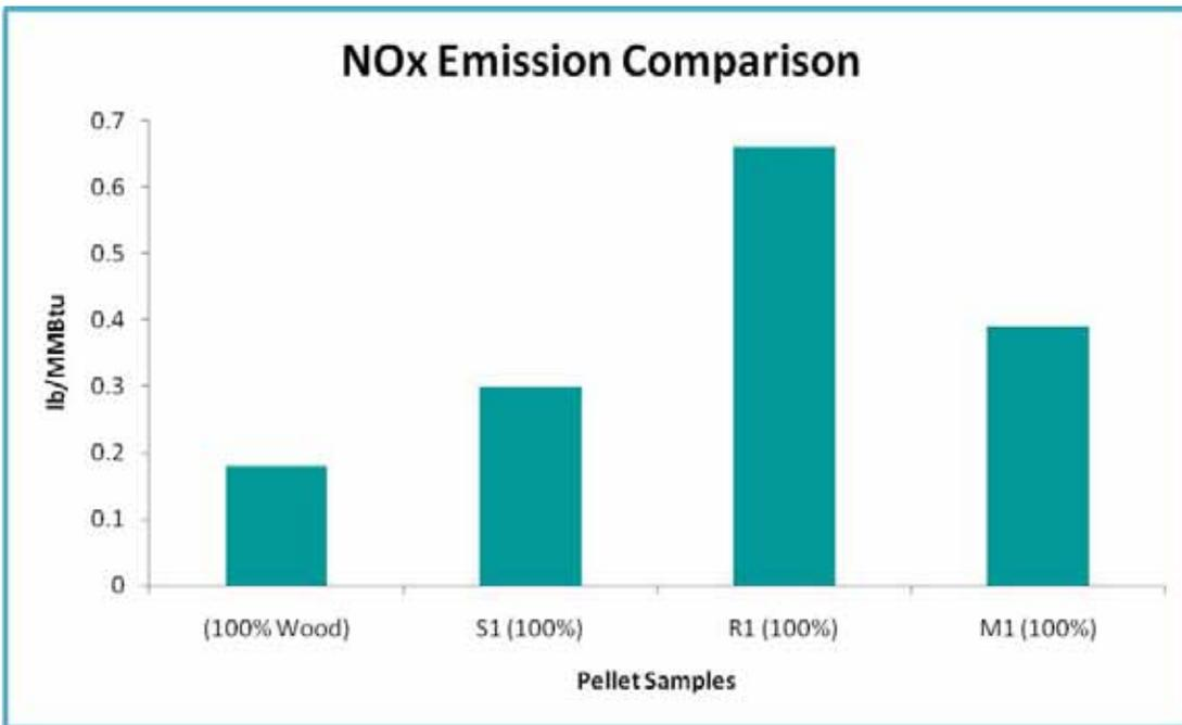
**While there are no cost-effective back-end control technologies for NO<sub>x</sub> for systems smaller than 15 MMBtu/hour, there are such control technologies for larger systems.**
