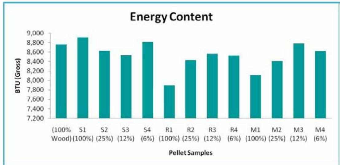
the control wood pellet and the grass/wood blends with more wood fiber content. While this data indicates switchgrass pellets have slightly higher energy value than pelletized wood, most data suggests that switchgrass pellets normally have slightly less (2-3%) than wood pellets.<sup>9</sup> This inconsistency does not present a problem due to the relatively slim margin of difference of energy content between the S1 and control wood pellet samples.
